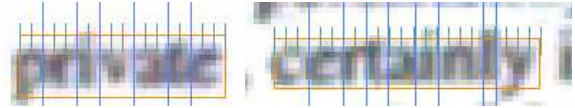
Figure 2. Word segmentation. The small (green) hash marks indicate the slice size for segmenting a word. The long (blue) hash marks indicate the slices actually used for each of the letters in the words "private" and "certainly".
