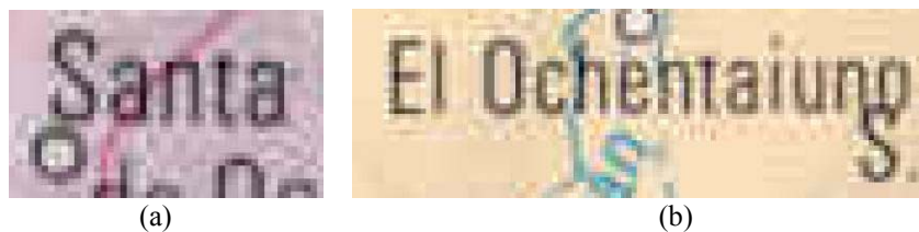
Fig. 5. (a) Character touching a symbol with similar features; (b) Character overlapping two characters with identical features
