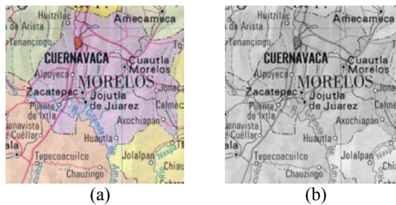
Fig. 1. (a) Example of color cartographic map with different types of characters; (b) Gray-level image ( Y-luminance ) corresponding to the image of Figure 1
