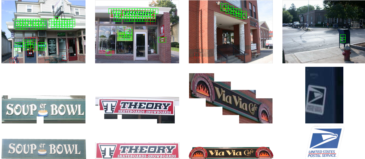
Figure 8. Four sample results of the integrated system. The top row is an image scene; green (solid) boxes mark detected sign regions and red (dashed) are false positives. The second row is a set of connected, detected patch components that are passed to the recognition system. The third row shows sign classes successfully recognized.
